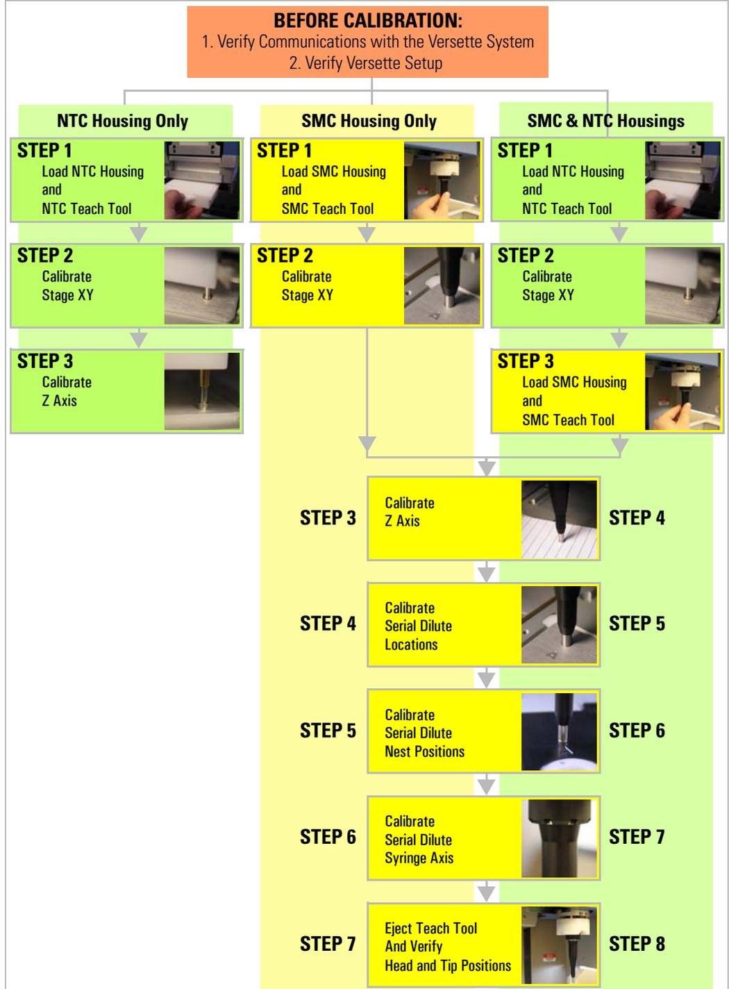
Figure 14. Versette Calibration Master Flowchart
