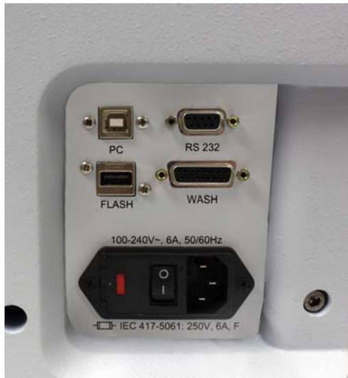
2. Connect supplied power cable to the system and to a correctly installed line power outlet which has a protective conductor, also called earth or ground.
