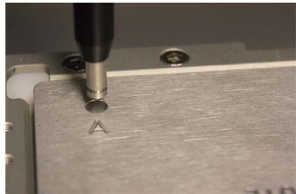
5. Check the alignment location. The teach tool should be positioned in the exact center of the Calibration Plate left rear hole marked "A".
