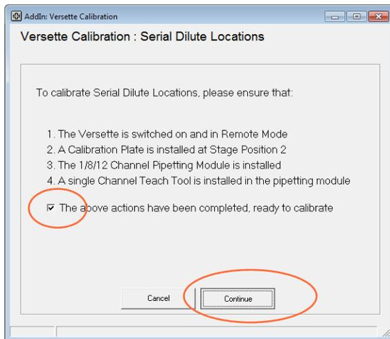
3. The Serial Dilute coordinates are calibrated from Stage 2. Select Stage 2 from the drop-down menu, then click “**Move to Position**”.
