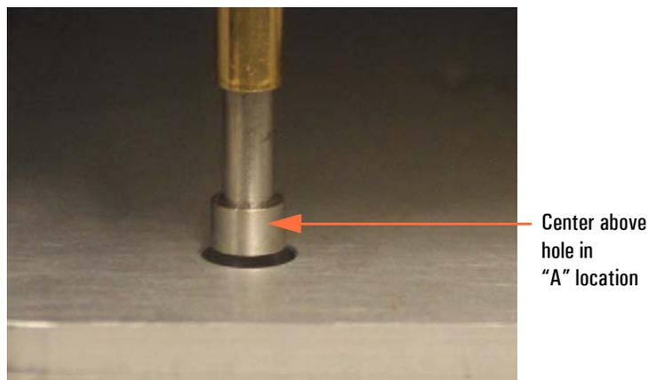
8. Lower the pipetting module slightly to verify that the X-axis and Y-axis alignments are properly set. Take care to check the left rear hole and the right front hole marked as “A” locations on the Calibration Plate.
