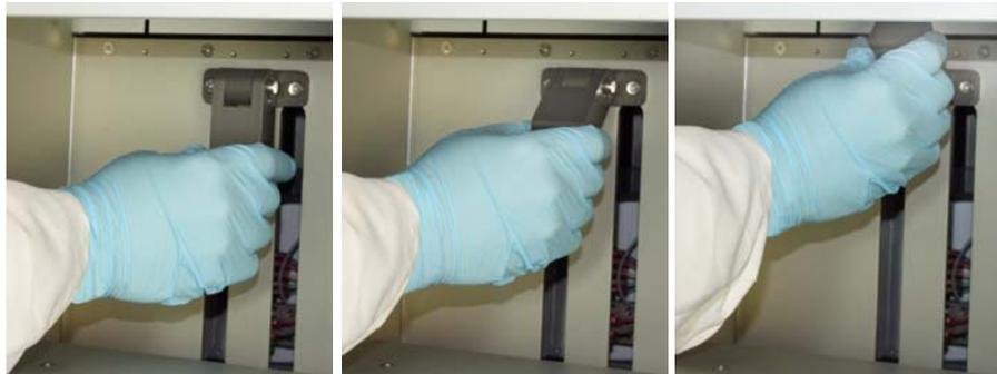
Rotate Release Bar to UP position.
