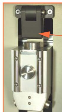
Rotate Release Bar to point down
