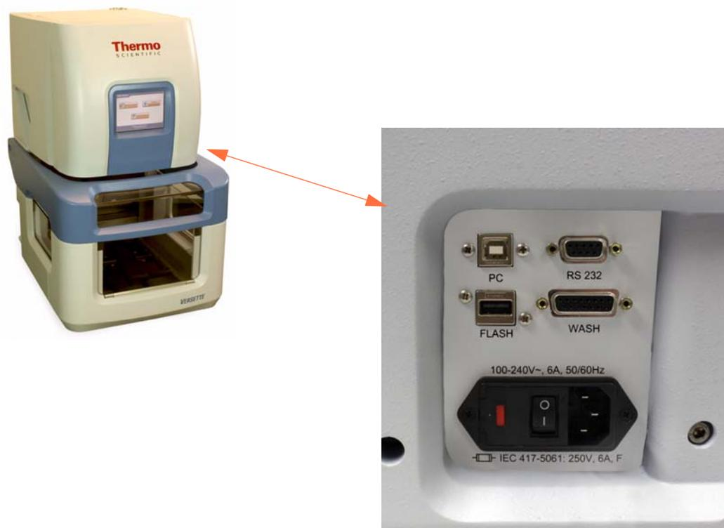
Figure 6. Versette, Power/Communications Connections, Right Side of Unit
