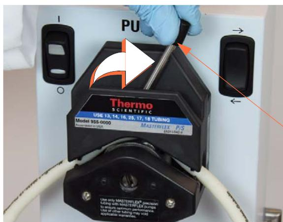
Rotate clamp lever to right side to lock tubing in place
