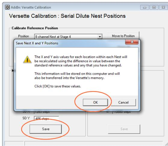
6. Wait approximately 15 seconds for the system to save the changes. Do NOT close the window! The window will close automatically and return to the Calibration Menu.
