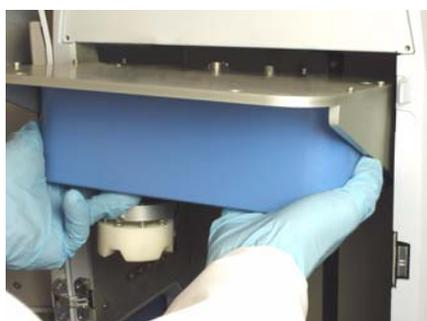
SMC Pipetting Module installation
