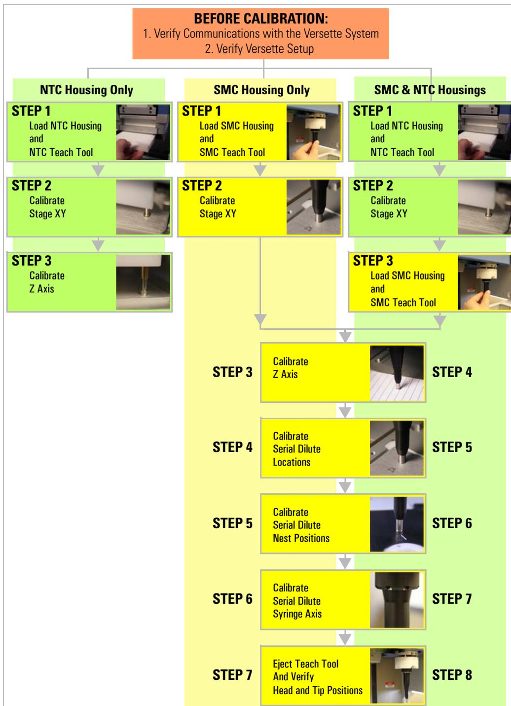
Figure 16. Versette Calibration Master Flowchart
