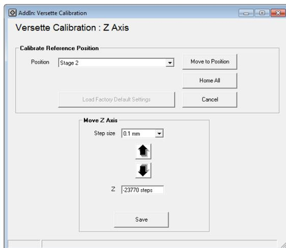
7. Try to gently pull the paper out from under the Teach Tool. If you can move the paper, lower the teach tool again by 0.1 mm then check again. Continue this until you cannot pull the paper out from under the Teach Tool.
