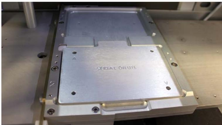
Press the plate firmly down in place to ensure that it is absolutely flat, firmly positioned in the stage.
