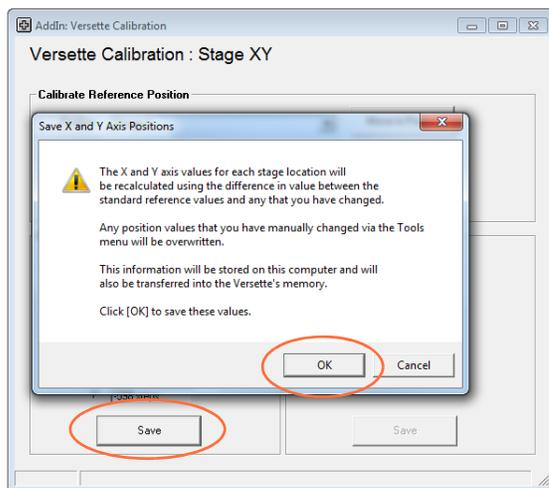
10. Wait approximately 15 seconds for the system to save the changes. Do NOT close the window! The window will close automatically and return to the Calibration Menu.
