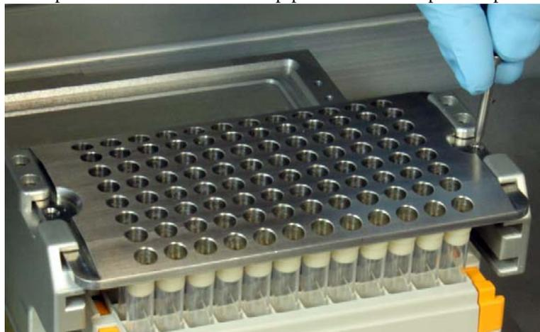
6. Install an appropriate piercing head, and use the onboard or ControlMate software to program operation.
