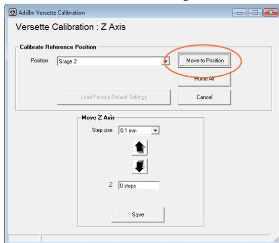
4. Set the **Step size**, then use the arrows to move the teach tool down until it is close to the Calibration Plate, as shown below.
