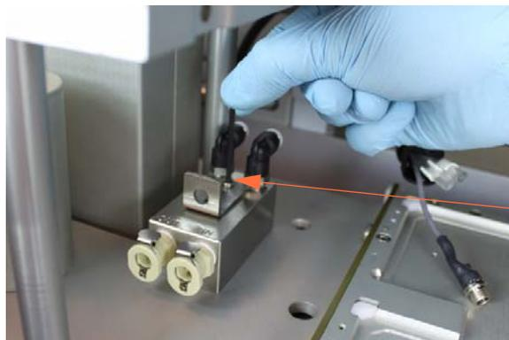
Connect to base of stage with 2 M3 screws, supplied
