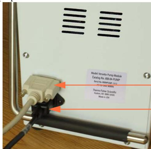
Connect 15-pin communication cable to the pump module
