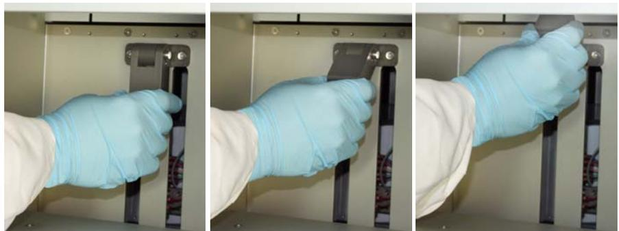
Rotate Release Bar to UP position.
