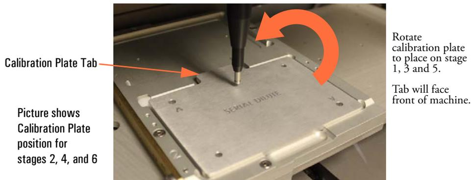
c. Use the dropdown box to select the stage where the Calibration Plate is installed, then click **“Move to Position”**. The unit will go through a homing cycle, then move to the selected stage position.
