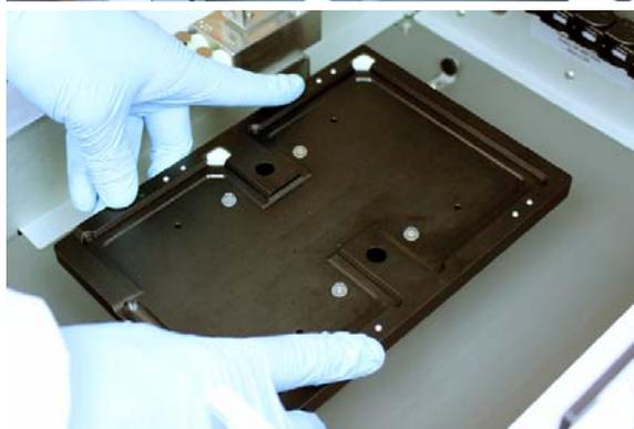
Seat 4 corner guideposts firmly on stage platform
