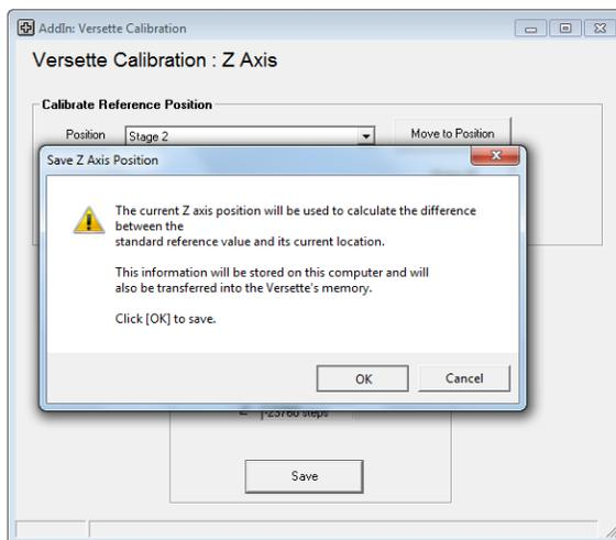
10. Wait approximately 15 seconds for the system to save the changes. Do NOT close the window! The window will close automatically and return to the Calibration Menu.
