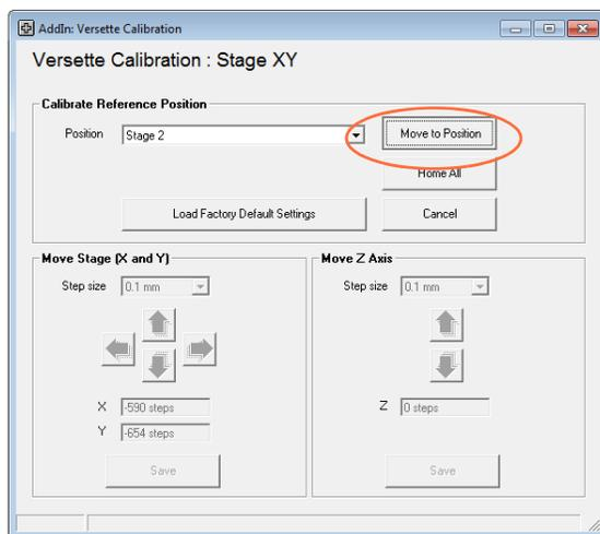
6. After Stage 2 has moved in position under the teach tool, use “Move Z Axis” to lower the teach tool to approximately 1 mm above the Calibration Plate.
