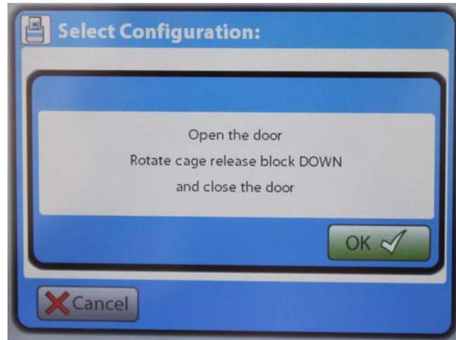
4. Rotate the pipetting module release block to the down position, then close the door and press "Next." Note: The door interlock prevents motion with the door open.
