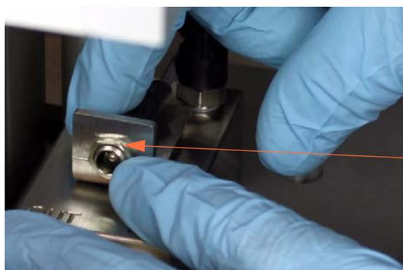
Connect tubes as labeled, then connect cable with nut, supplied
