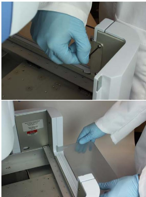
2. Remove top shield and install top of waste bin shielding.
