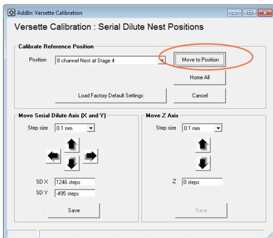
4. Carefully evaluate the position of the Teach Tool alignment. If necessary, select the **Step size** (0.1mm, 1mm, 10mm, etc.), then use the arrows to precisely align the teach tool in the alignment hole, as shown.
