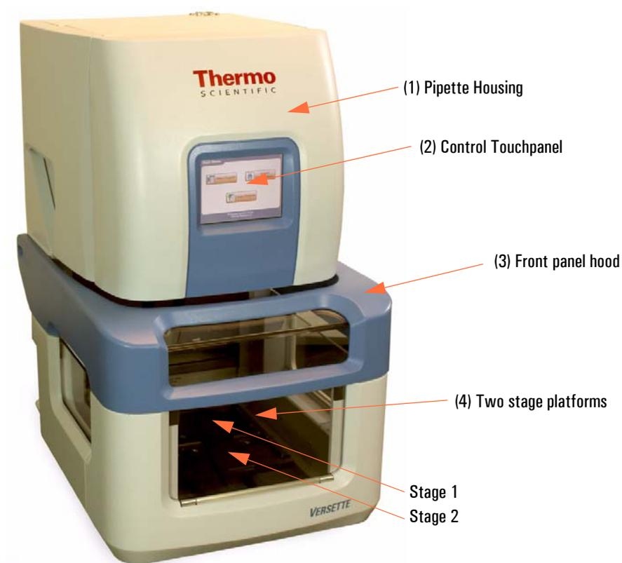
Figure 4. Thermo Scientific Versette Components 2-Stage System- Front View
