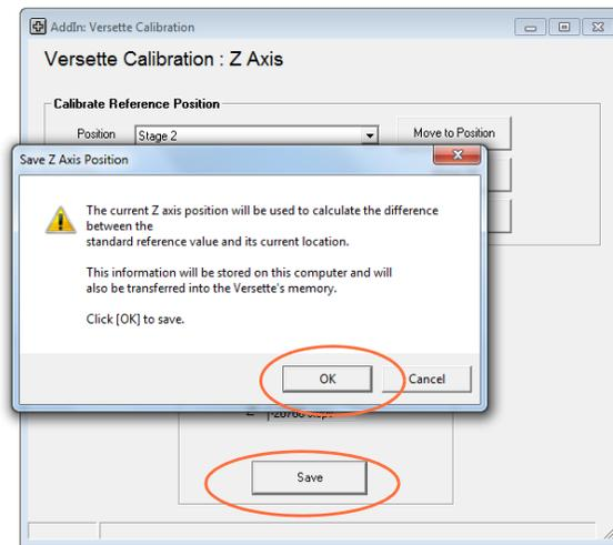
6. Wait approximately 15 seconds for the system to save the changes. Do NOT close the window! The window will close automatically and return to the Calibration Menu
