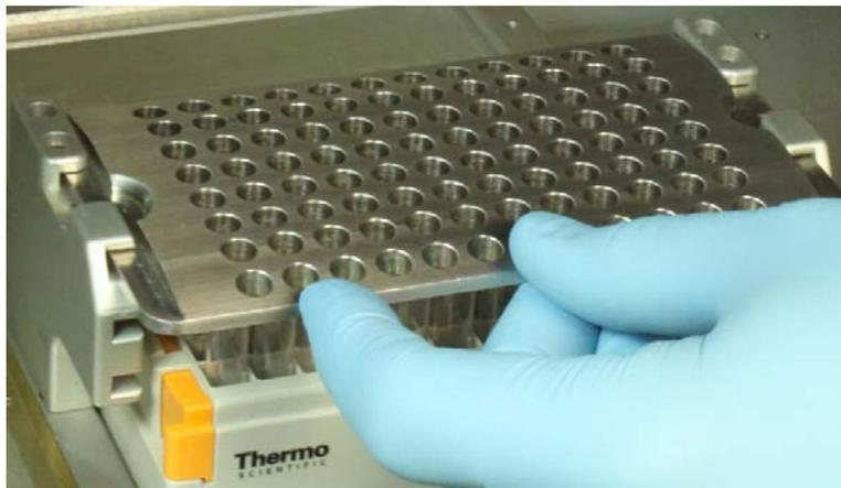
5. Insert pins into each side of the top plate to hold the plate in position.
