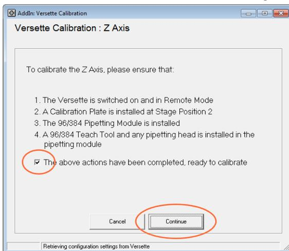
3. The Z-Axis is calibrated from Stage 2. Verify that Stage 2 is displayed in the position box, then press “**Move to Position.**” The head and stages will move to position the Teach Tool over the Calibration Plate on Stage 2.
