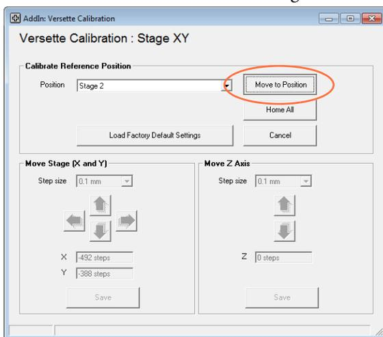
6. Set the **Step size**, then use the arrows to move the teach tool down until it is close to the Calibration Plate, as shown below.
