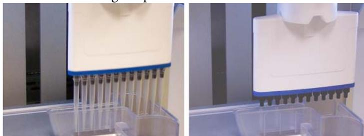
1) Head moves over and into tip transfer chute
