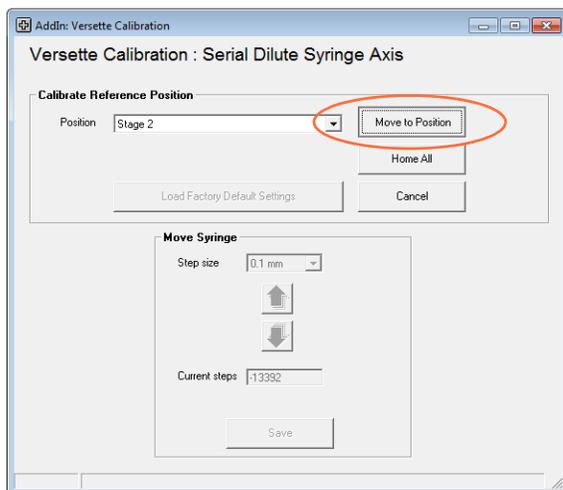
4. Use the **Step size** and arrows to move the teach tool until the silver ring is positioned as shown in the final alignment photograph below.
