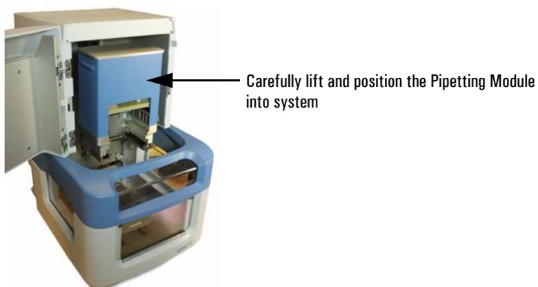
NTC Pipetting Module installation
