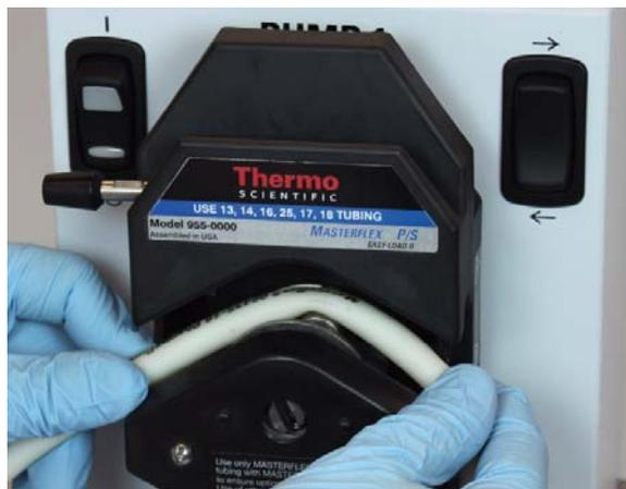
4. Push tubing all the way into the system. Be sure to push the tubing all the way into the clips on each side, as shown.
