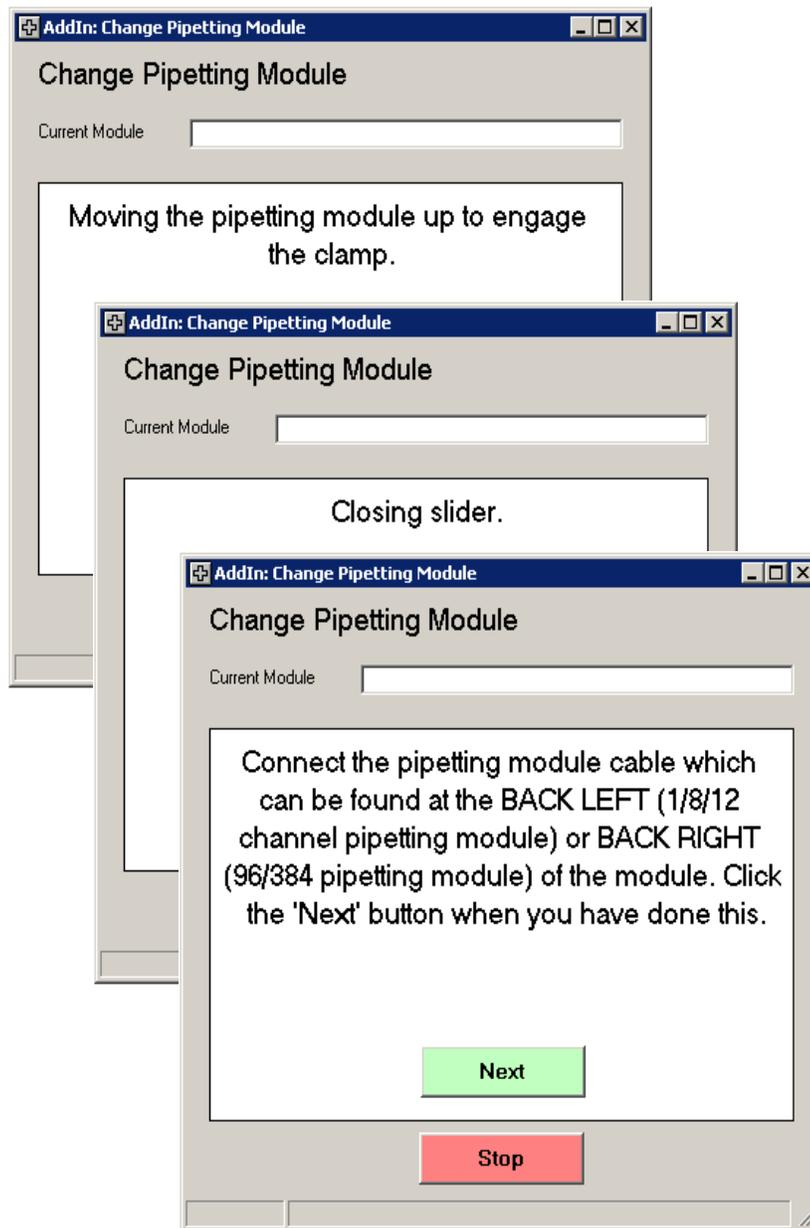
The cable connector may have red dots which align to the system connector. The dots are difficult to see due to their location. Follow the screen messages carefully and press in firmly to ensure proper connection.
