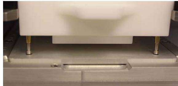
7. Check the alignment location. The teach tool posts should be positioned in the exact center of the Calibration Plate holes. Alignment of the holes marked "A" (left rear, and right front) is critical.
