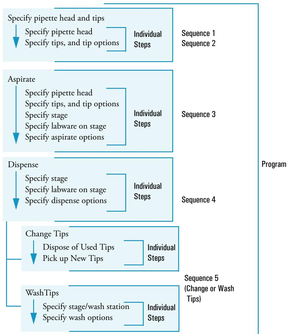
Figure 11. Sample basic program components
