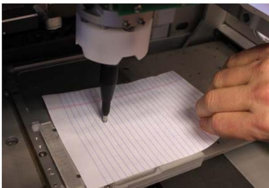
8. When you cannot move the paper out from under the Teach Tool, RAISE the Teach Tool by 0.1 mm. (One press of the up button.)
