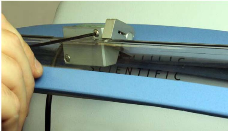
3. Adhere wire clips to the underside of the shield (if needed) and feed the wire out the rear of the system, as shown.
