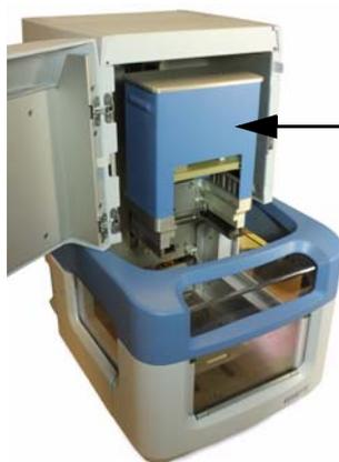
Carefully lift and position the pipetting module into the system
