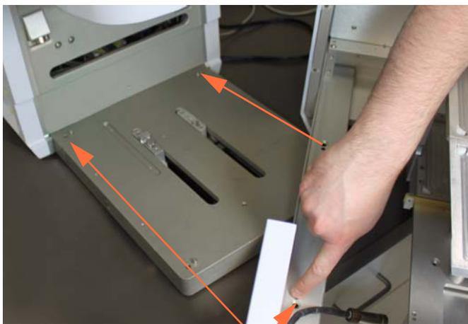
Align 4 corner holes and alignment posts
