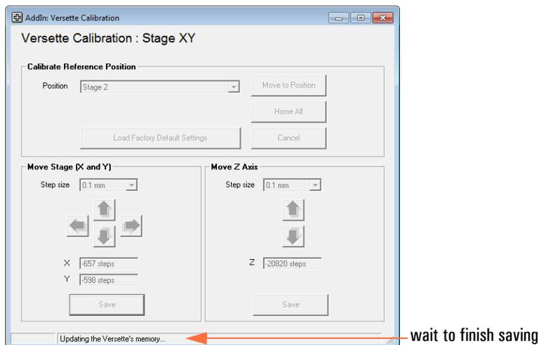
11. OPTIONAL: Verify the accuracy of calibration at each remaining stage location, as detailed below. If no changes are made on a specific stage, there is no need to click save, just move to the next location and continue to check each stage position.
