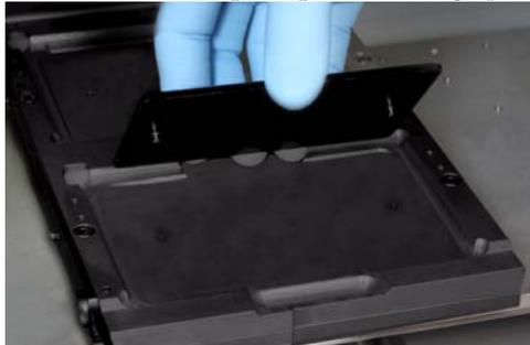
2. Attach side brackets to stage position. Optional extenders with longer screws are provided.
