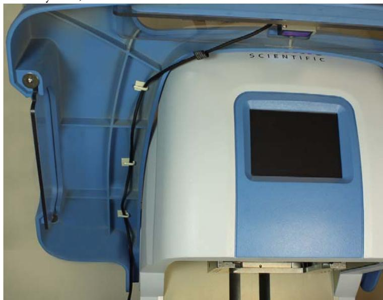
4. Connect the barcode reader cables, per instructions provided with the barcode reader.
