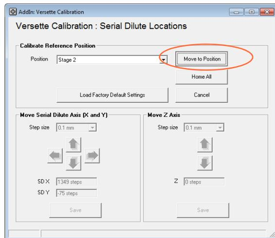
4. After the system has stopped moving, use “Move Z Axis” to lower the head down to approximately 1 mm above the Calibration Plate.
