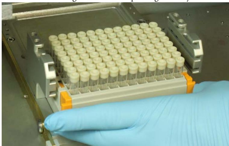
4. Slide the top plate over the tubes. The brackets have multiple slots for short and long tubes.
