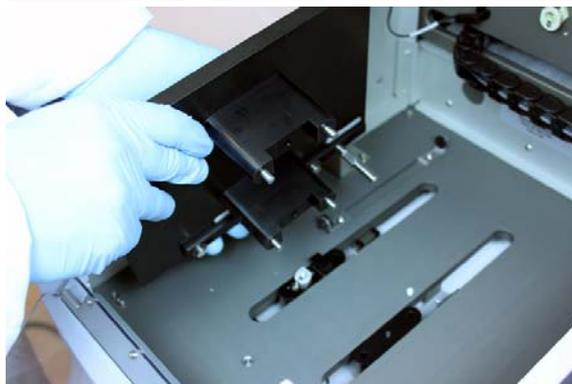
Place stage in system with long guidepost at left-rear to slide between bumpers on stage base
