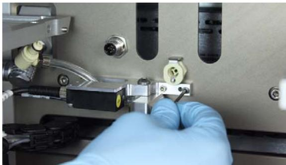
2. Connect fill tube to N/C fill connection on backplane.
