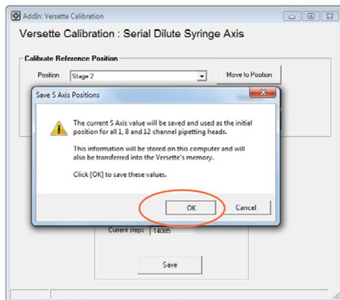
8. Wait approximately 15 seconds for the system to save the changes. Do NOT close the window! The window will close automatically and return to the Calibration Menu.
