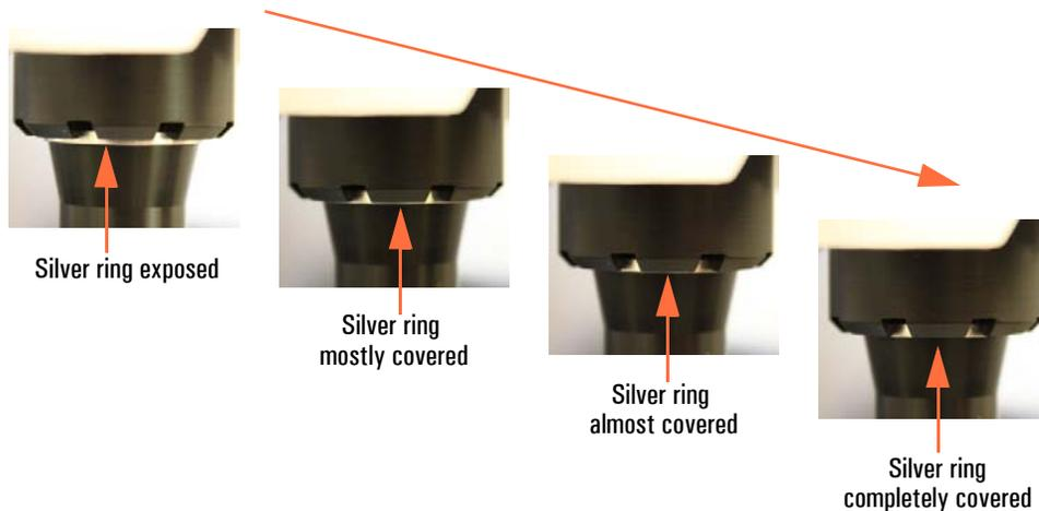
5. When precisely positioned, click **Save**. The system will verify the calibration position. Wait for the screen prompts.
