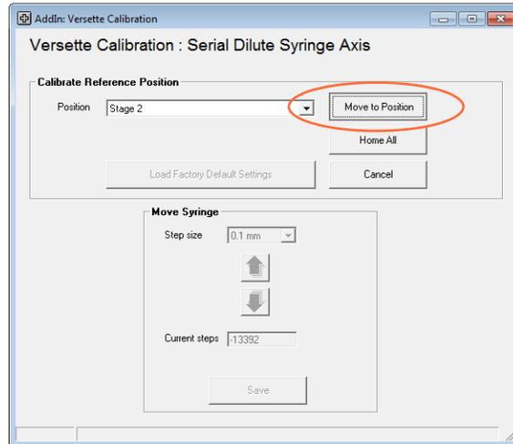
4. Use the **Step size** and arrows to move the teach tool until the silver ring is positioned as shown in the final alignment photograph below.
